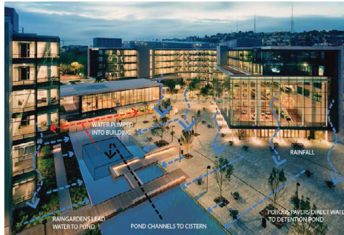
Diagram illustrates how stormwater flows around the building. Image from NBBJ Architects; Diagram by Olivia
