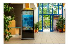
Soofa signs are sustainable, solar-powered digital signs. They are 7.5 feet tall and contain a 42-inch electronic ink display. The screen is in two sections; the top 75 percent can update every two minutes,
