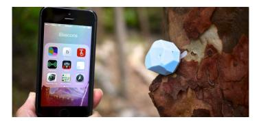
Beacons are Bluetooth radio transmitters. They constantly release signals to Bluetooth-enabled devices within range—typically about 50 meters/160 feet. Users download a corresponding app and enable their Bluetooth service to receive beacon notifications. Beacons are typically used for marketing purposes but can be used to convey any type of information.
